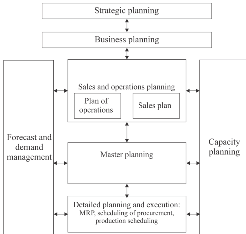
Figure 2. Architecture of business processes of ERP system
